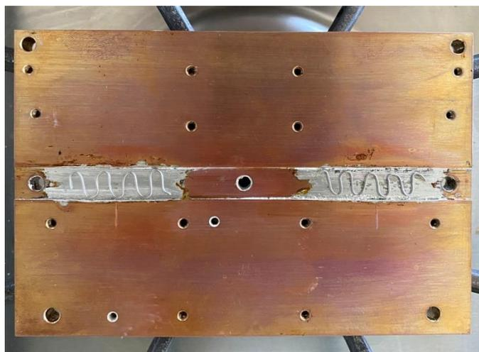
Figure 2 - heat spreader with old solder removed, new solder in the trench
