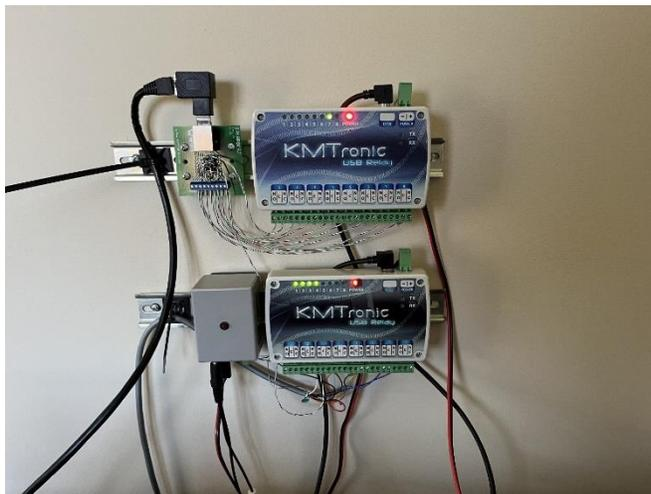
Figure 4 Control switches in shack. Top is RX control, bottom is other antennas
