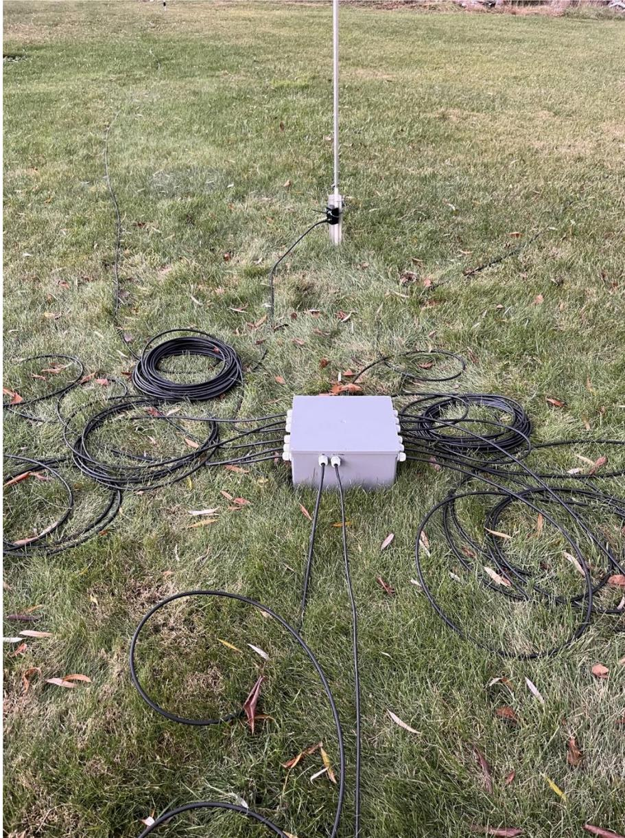
Figure 3. Combiner deployed, coax and center element.
