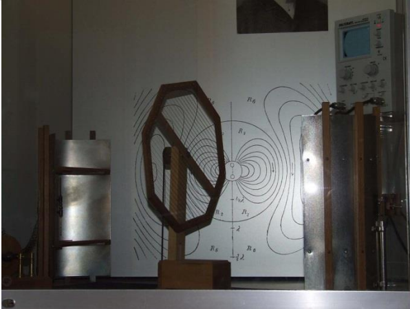
Heinrich Hertz's experiment, which took place in 1886, demonstrates the existence of radio waves and their polarity.
