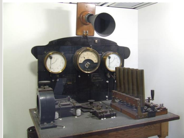
In 1906 the first radio transmission of speech was performed using a sound-modulated arc transmitter. The microphone is fed directly into the antenna circuit.
