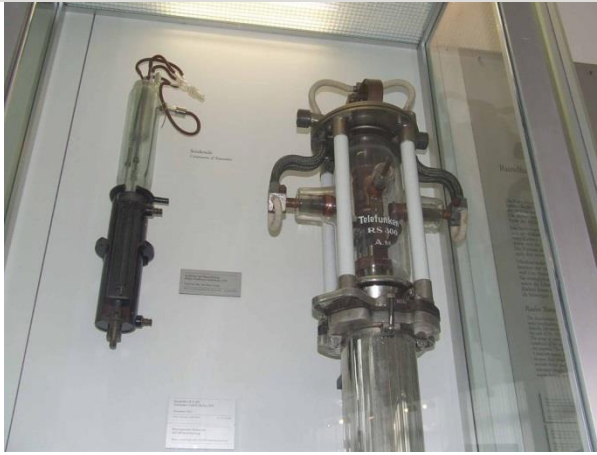
A Philips water-cooled transmitter tube from 1924 with a 300 kW Telefunken water-cooled tube (right). The name Telefunken itself is a tribute to spark-gap transmitters: "funken" in German means "sparks."
